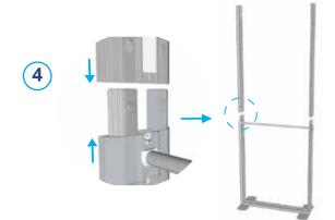
Attach the top vertical profile components to the straight connectors
