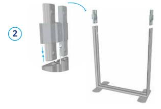
Align the vertical profile extrusions with the straight connector and push them together until securely slotted into one another.
