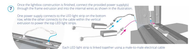
(up to three LED light strips can be connected from one power supply)
