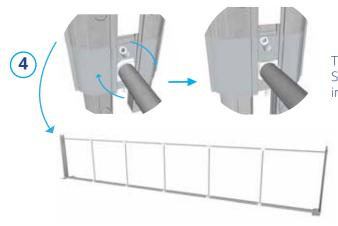
To enhance stability, incorporate horizontal and vertical support poles. Slot them together by rotating into the grooves of the straight extrusion, including when inserting into the centre cross connector.
