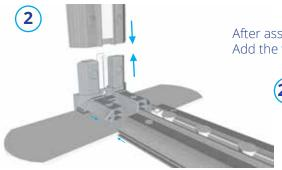
After assembling the base, join the feet by pushing them together until they click. Add the vertical profile extrusions by connecting it to the feet.
