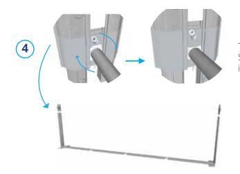
To enhance stability, incorporate horizontal and vertical support poles. Slot them together by rotating into the grooves of the straight extrusion, including when inserting into the centre cross connector.
