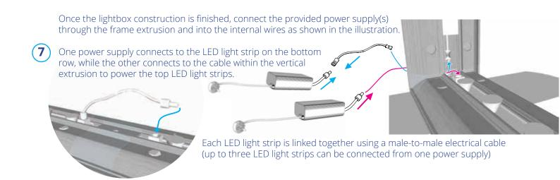
Once all wires are connected and plugged in, insert your chosen fabric graphic to finish your lightbox display.
